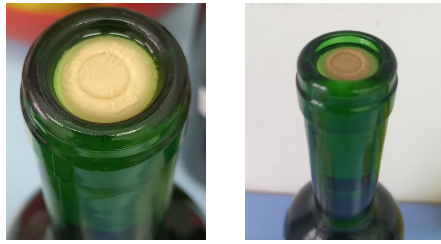
Figure 6 A faulty stopper
