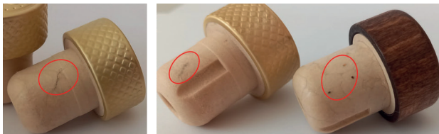
Figure 22 Contamination on the surface of T-shape polymer stoppers
