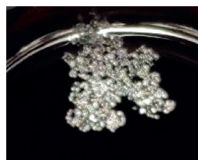
Figure 16 Foreign inclusions on cognac surface, 100× magnification
