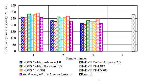
**Fig. 3.** Effective dynamic viscosity of yogurt samples (at the share rate of 300 s<sup>-1</sup>).
