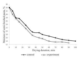
Fig. 3. Drying curves for semi-finished pasta.
