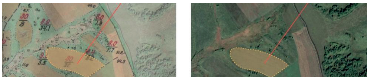
Figure 1 Faulty boundaries revealed by comparing a digitized paper map with the aerial photography data
